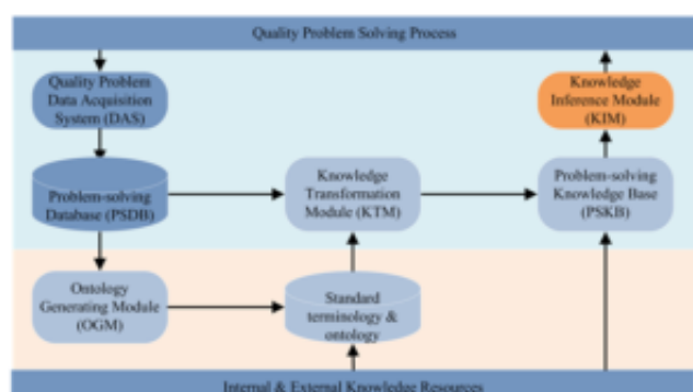
Figure 3. The architecture of knowledge management based intelligent problem-solving system (IPSS).
